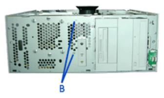
Figure 4 - 19: HDD Bracket Screws
